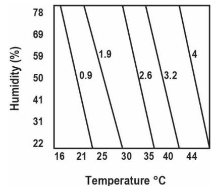
**Figure 2: Cure in depth after 24 hours.**
